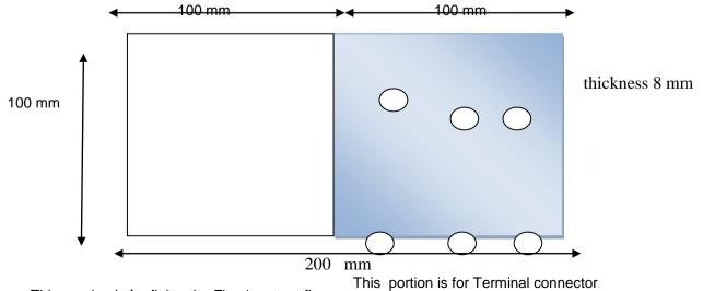
This portion is for fitting the Fixed contact finger
